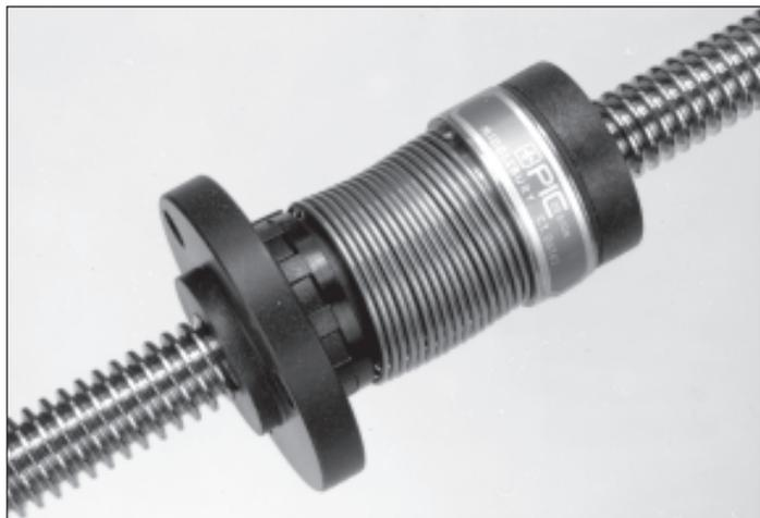
PV style anti-backlash nuts provide a maximum load carrying capability and the lightest axial and radial stiffness of all PIC anti-backlash nuts. They are designed for smooth, quiet operation and long life, made possible by a patented axial take-up mechanism. Because this series is designed to operate with higher loads, operation is only possible with 1/2" and 3/4" diameter lead screws.
